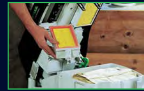
No tools needed to change the HEPA or flat filters
